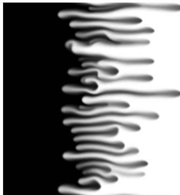
FIGURE 2. Numerical simulation of miscible viscous fingering (defined in (1.1)–(1.3)) from Booth (2008), with a constant flux of solvent (on left of image) into oil, and M = 5 , Pe = 3000 . Numerical simulation uses a high-resolution finite-volume method with flux limiters.
